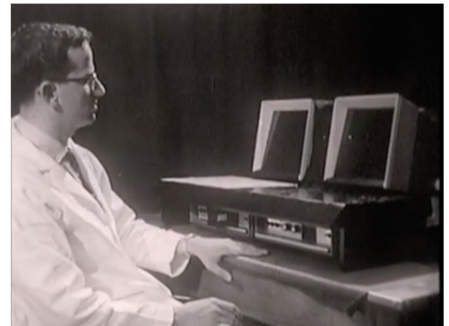
Mike Gazzaniga at Cal Tech with one of the first tachistoscopes used to lateralize visual stimuli to a single hemisphere
