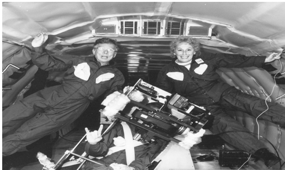
Markham and Diamond experience zero gravity during parabolic flight as they collect eye movement data from a participant (center) to develop a predictive test for space motion sickness..
